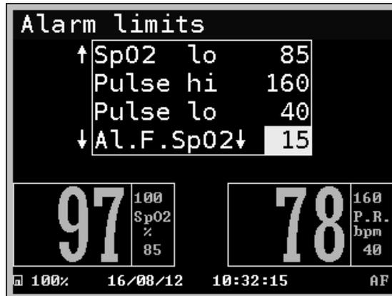
**Fig. 35: Modifying the alarm filter**
