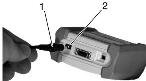
**Fig. 4: Plug adapter cable into socket**
