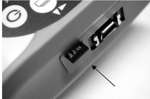
Fig. 62: Inserting SD card
