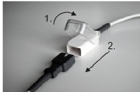
Fig. 18: LNCS sensor coupling
