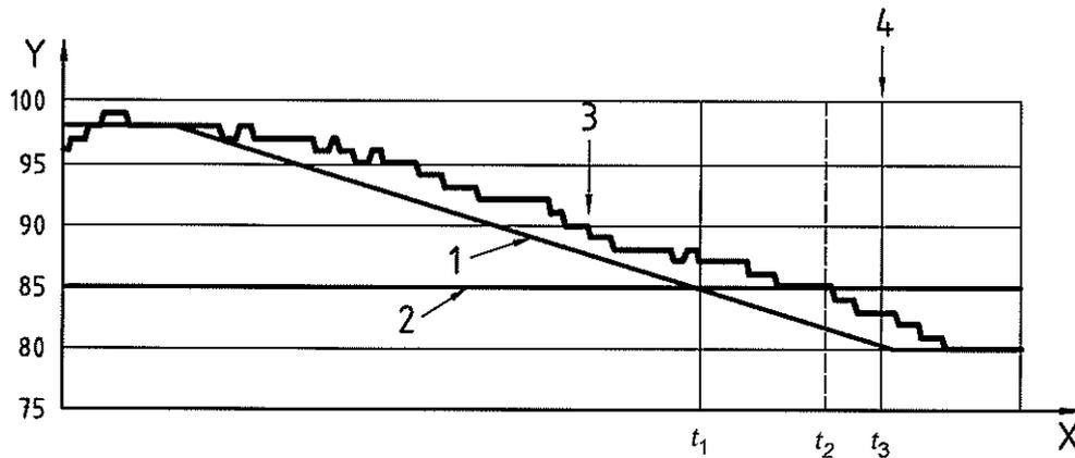
The delay due to the pulse oximeter equipment processing and averaging is  $t_2 - t_1$ , the alarm condition delay. The interval  $t_3 - t_2$ , the alarm signal generation delay, is attributed to the alarm system strategy and the communication time to the alarm signal generation device or distributed alarm system (e.g. patient monitor or central station). Thus, the overall alarm system delay time is  $t_3 - t_1$ .
