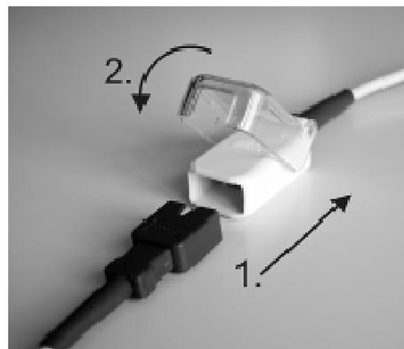
**Fig. 16: LNCS sensor connection**
