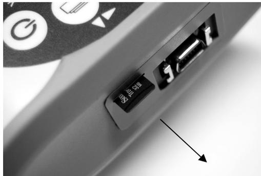
**Fig. 64: Removing the SD card**
