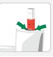
**NOTE:** Create vacuum to green section on gauge. If possible, 'burry' the green so it is no longer visible.
