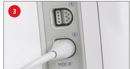
3 Connect the O 3 MOC-9 module to one of three Root MOC-9 Ports.
