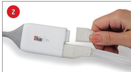
2 Connect the O 3 sensors to an O 3 MOC-9 module (up to two sensors per module).
